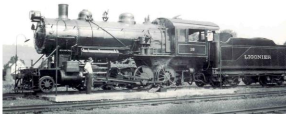
Engines with the 2-8-0 wheel configuration, as seen in this photograph of Engine #18, were designed for pulling power.
